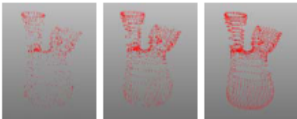
Fig. 2.2: Results from curvature sampling on the surface model at (from left) 30% curvature sample, 65% curvature sample and 100% curvature sample.
