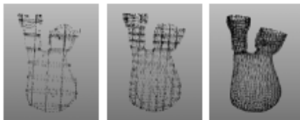
Fig. 2.3: Results from polygonal surface reconstruction (from left) at 10mm, 5mm and 2mm point distance.
